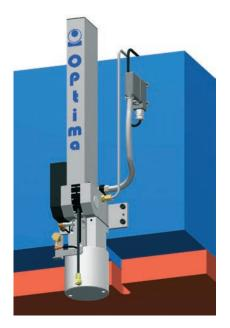
Fixing is achieved with four hexagon head screws with flange (DIN 6921), M10x30, strength class 8.8 and two spring dowelpins (DIN 1481) Ø8x20 (not included).
